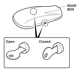
**Locking**: Press down on the lid. There should be an audible click. Be sure the lid is latched by attempting to lift the lid. Turn the key clockwise to lock the roof box. Be sure the straps are not outside of the roof box.
