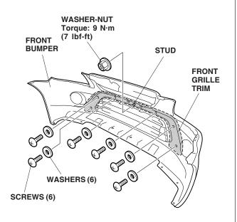
10. Reinstall the front bumper and radiator cover. If equipped, plug in the fog light connectors.
