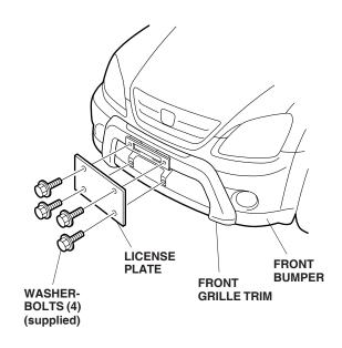
11. Install the license plate on the front grille trim with the four washer-bolts supplied.
