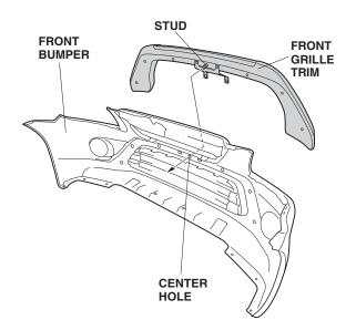
Install the washer-nut on the end of the stud, then install one screw with washer through the remaining six holes and into the front grille trim. Torque the washer-nut to 9 N·m (7 lbf-ft).
