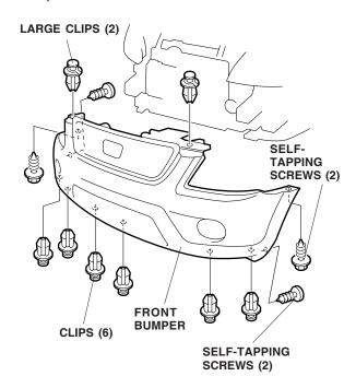
3. Inside the front bumper, cut off the two pins, and remove the push nuts and the old "H" emblem.
