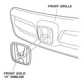
5. Slide the push nuts onto the pins. Note the direction of the push nuts.
