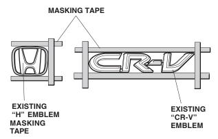
8. Remove the "H" and "CR-V" emblems from the body by moving the string back and forth, working it between the emblems and body.
