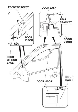
Adjust the location of the door visor so that the clearance between the door visor and door sash is 2 mm at the top, and 3 mm at the back. There should be no clearance between the front tab and the visor.
