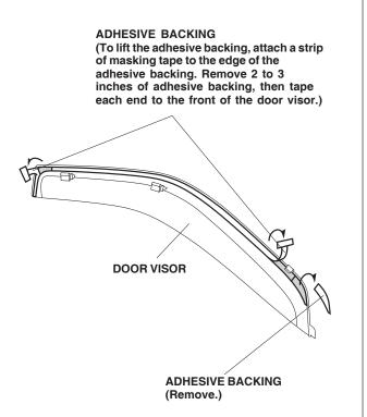
4. Attach a strip of masking tape to the ends of the two remaining adhesive backing pieces, and remove 2 to 3 inches of adhesive backing. Fold back the ends, then tape the ends to the front of the door visor. Note the removal direction of the adhesive backing.
