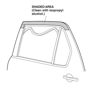
11. Attach a strip of the masking tape to the ends of the three adhesive backing pieces, and remove 2 to 3 inches of adhesive backing. Fold back the ends, then tape the ends to the front of the door visor. Fold the ends back then tape them to the door visor. Note the removal direction of the adhesive backing.
