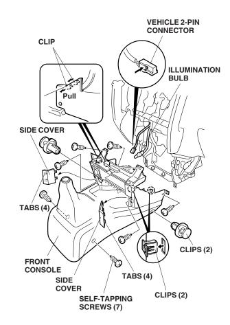
12. On M/T vehicle only, remove the two clips and seven self-tapping screws, and pull the front console out toward you to release four clips. Unplug the 2-pin connector from the accessory socket, then remove the front console. 13. Open the lid on the cigarette lighter. Using a shop towel around a flat-tip screwdriver, gently pry on the socket, then remove the case.
