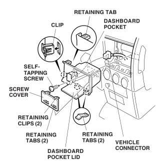
Remove two self-tapping screws that fasten the heater A/C control panel to the dashboard. Pull the heater A/C control panel out toward you to release the four clips. Unplug the vehicle connector, then remove the heater A/C control panel.
