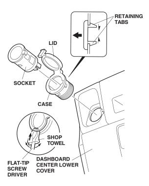
14. Slide the ring into the hole in the dashboard center lower cover in the direction shown.
