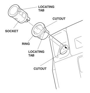
15. Align the locating tab of the socket with the cutout in the ring, then slide the socket of the cigarette lighter into the ring.
