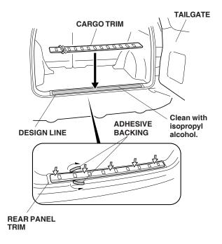
Attach the cargo trim by removing the adhesive backings. Hold pressure on the rear panel trim for 30 seconds.
