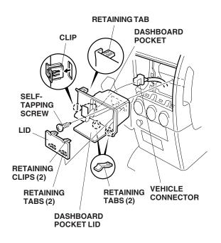
7. Remove the dashboard pocket (one self-tapping screw, one clip, three retaining tabs then unplug the vehicle connector).
