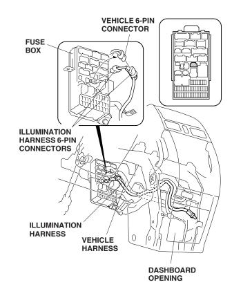
15. Route the illumination harness to the dashboard opening along the vehicle harness.
