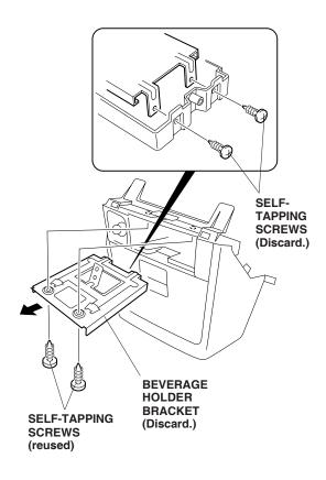
12. Remove the bracket from the ashtray, then install the bracket on the dashboard center lower cover using the two self-tapping screws you just removed and one self-tapping screw supplied.
