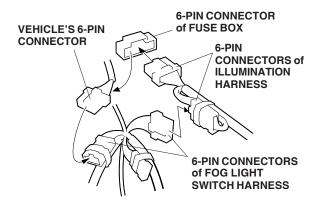
16. Secure the illumination harness to the vehicle harness with four wire ties.
