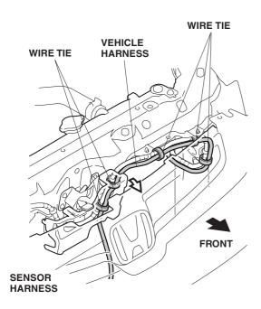
12. Near the battery, continue routing the sensor harness along the vehicle harness, and secure it to the vehicle harness with four wire ties.
