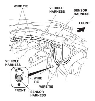
13. Lift the air cleaner housing cover upward, and route the sensor harness toward the rear along the vehicle harness.
