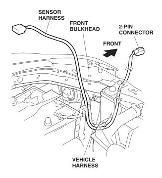
10. Push the sensor harness clip into the hole on the sensor bracket.
