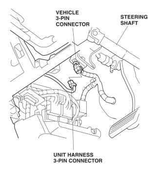
NOTE: If the 3-pin connector is already being used by another accessory, locate the 3-pin connector taped to that other accessory's harness. Remove the dummy connector from that other accessory's harness. Plug the unit harness 3-pin connector into the other accessory's harness.
