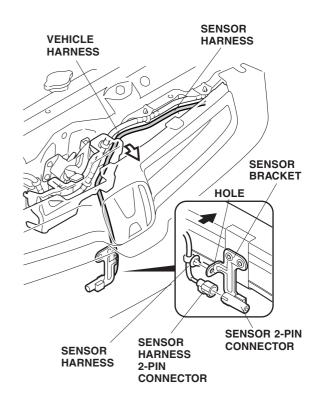
11. Pull hood lock cover, and secure the sensor harness to the vehicle harness with the five wire ties in the areas shown.
