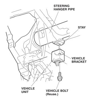
24. Combine the vehicle bracket and the unit bracket, install them to the stay on the steering hanger pipe with the vehicle bolt (reused), and slide the unit bracket onto the control unit.
