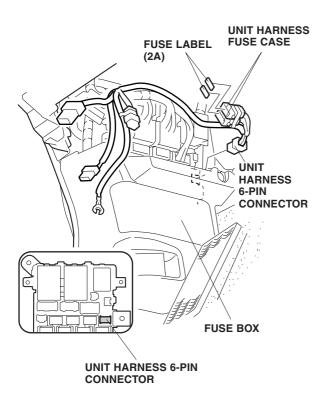
20. Plug the 6-pin connector of the unit harness into the fuse box.
