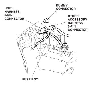
21. Loosen the vehicle ground bolt, and install the unit harness ground terminal with this bolt.
