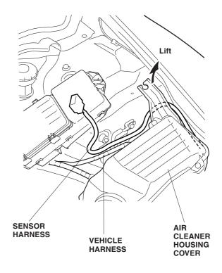
14. Under the relay box, locate the vehicle 3-pin connector blue-taped to the vehicle harness, and remove the blue tape to free the connector. Connect the sensor harness 3-pin connector into the 3-pin connector you just freed. Secure the sensor harness to the vehicle harness with wire ties in the areas shown.
