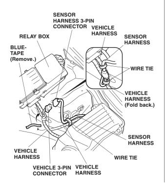
NOTE: If the 3-pin connector is already being used by another accessory, locate the 3-pin connector taped to that other accessory's harness. Remove the tape and dummy connector from that other accessory's harness. Plug the sensor harness 3-pin connector into that other accessory's harness.
