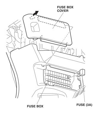
18. Attach the fuse label (3A) over the No. 33 on the back of the fuse box cover.
