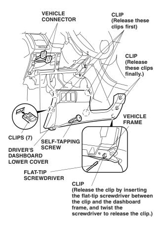
16. Remove the driver's dashboard under cover (release the three retaining clips, one pin and one holder).
