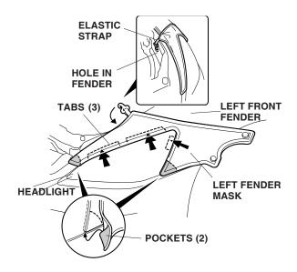
9. Pull the fender mask back toward the wheelwell, smooth out any wrinkles, and snap the fender mask onto the snap-screws.
