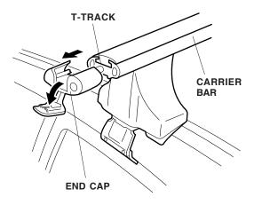
10. Remove the rubber moldings from the T-tracks of the front and rear carrier bars. Retain the rubber moldings to be installed later.
