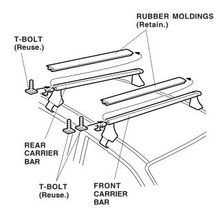
11. Slide two T-bolts into the front carrier bar, and slide one T-bolt into the rear carrier bar.
