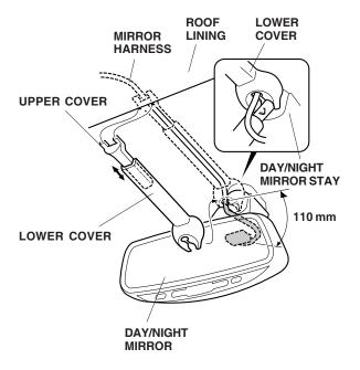
Remove the dummy connector from the vehicle harness 3-pin connector, then connect the vehicle harness 3-pin connector to the mirror harness 3-pin connector.
