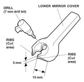
While wearing eye protection, drill a 7 mm hole through the existing hole on the lower cover as shown. 10. Measure and mark the mirror harness 110 mm from the 7-pin connector. Slide the end of the upper cover into the lower cover, then route the mirror harness through the grooves in the covers. Attach the lower cover to the mirror stay, and slide the upper cover to the edge of the roof liner.
