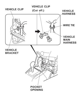
15. Cut off the vehicle clip and secure the vehicle harness to the vehicle main harness using a wire tie.
