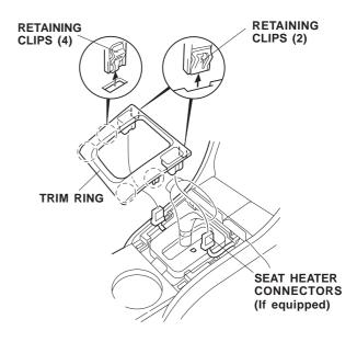
4. Remove the cup holder (pull up to release the six retaining clips).
