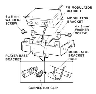
39. Install the player base-bracket into the holes in the vehicle frame.
