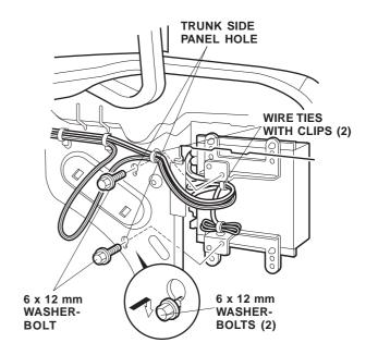
84. Fold any excess antenna cable, and wrap the excess cable with two EPT sealers. Secure the antenna cable to the XM radio harness with two wire ties in the areas shown. Tighten the off-set wire ties you loosely installed in step 77.
