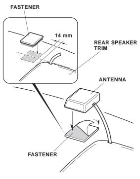
73. Route the antenna cable through the opening in the vehicle panel as shown.
