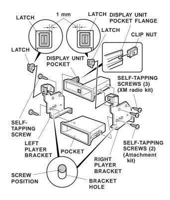
23. Set the display unit pocket on the pocket with the cutout facing up. Position the left and right player brackets on the display unit pocket and pocket, and install five self-tapping screws. Then go to step 26. 24. Install the latches onto the left and right player brackets. Slide the clip nut onto the display unit pocket flange
