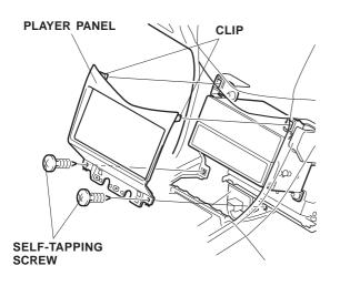
9. Remove the player/pocket assembly. Unscrew the four flange nuts, and pull the assembly out toward you. Unplug the audio bus cable connector.
