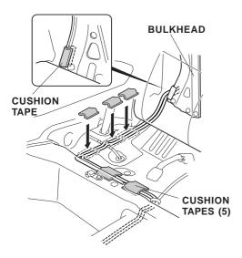
66. Using isopropyl alcohol, clean the bulkhead area where the cushion tape will attach. To prevent damage to the XM radio harness and DIN cable, attach the cushion tape to the bulkhead edge in the area shown. 67. Inside the trunk, install the two wire ties with clips to the DIN cable and XM radio harness, and push the clips into the holes in the bulkhead.
