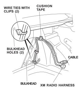
68. Using isopropyl alcohol on a shop towel, clean the area where the cushion tape will attach. Attach the DIN cable and XM radio harness to the vehicle frame with one cushion tape.
