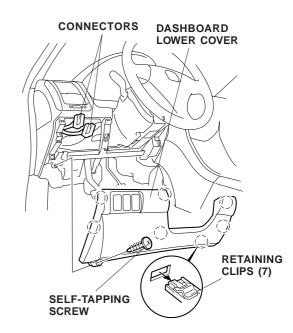
• If equipped, remove the driver's dashboard under cover (release the three retaining clips, one pin and one holder).
