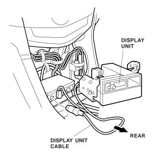
47. If equipped with a player, plug the bus cable connector into the vehicle connector.
