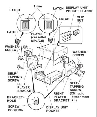
25. Set the player on the display unit pocket. Position the left and right player brackets on the display unit pocket and player, and reinstall the four washer-screws removed in step 10. Install the three self-tapping screws to secure the display unit pocket.
