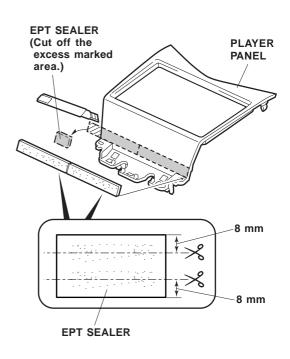
54. Using isopropyl alcohol on a shop towel, clean the player panel in the area shown. Attach the two cut pieces of the EPT sealer to the player panel, and cut off the excess.
