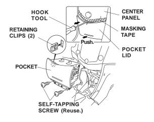
7. Remove the right and left inner covers (one hook and one clip for each cover). Set the inner covers aside; they will not be reused. Then go to step 11.
