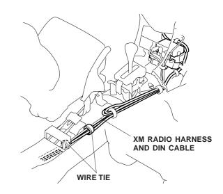
64. Raise the rear seat back. Pull the DIN cable and XM radio harness out past the edge in the floor carpet, then secure them to the vehicle harness with two wire ties.
