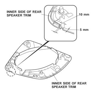
71. Route the antenna cable through the notch in the speaker trim, and install the rear speaker trim.
