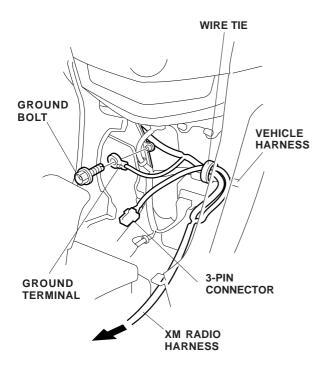
34. Secure the XM radio harness to the vehicle harness with one wire tie. Route the 3-pin connector and the remaining end of the XM radio harness toward the rear of the vehicle; they will be routed later.
