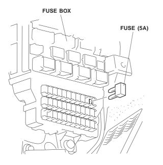
86. Attach the 5A fuse label over the No. 33 position on the fuse box cover.
