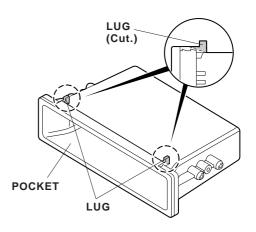
22. Install the latches onto the left and right player brackets. Slide the clip nut onto the display unit pocket flange.
