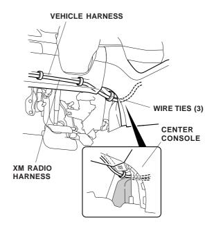
32. Attach the XM radio harness to the vehicle harness with three wire ties.
