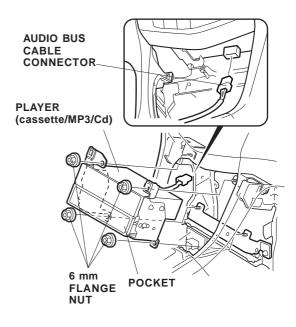
10. Remove the left and right audio brackets (two washer-screws and one self-tapping screw for each bracket). Separate the player and pocket. Set the pocket aside, it will not be reused.
