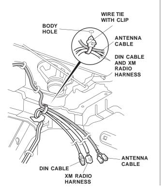
77. Route the antenna cable, XM radio harness and DIN cable along the trunk side panel, then loosely attach the three off-set wire ties with clips to the antenna cable, XM radio harness, and DIN cable, and push the clips into the trunk side panel at the three trunk side panel holes.
