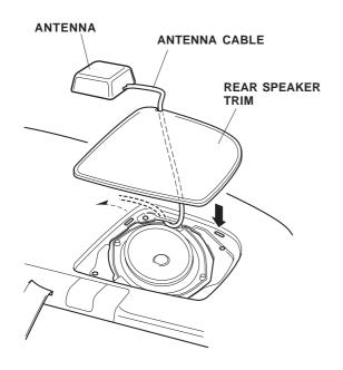
72. Using isopropyl alcohol on a shop towel, clean the bottom of the antenna. Remove the adhesive backing from the fastener, then attach the fastener to the bottom of the antenna. Attach the antenna onto the rear shelf.
