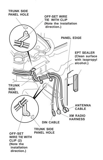
78. Using isopropyl alcohol on a shop towel, clean the bonding surface on the panel edge, then attach the EPT sealer to the panel edge in the area shown.
