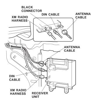
81. Secure the antenna cable, XM radio harness, and DIN cable with two wire ties with clips. Press the clips on the wire ties into the trunk side panel hole and upper unit bracket hole.
