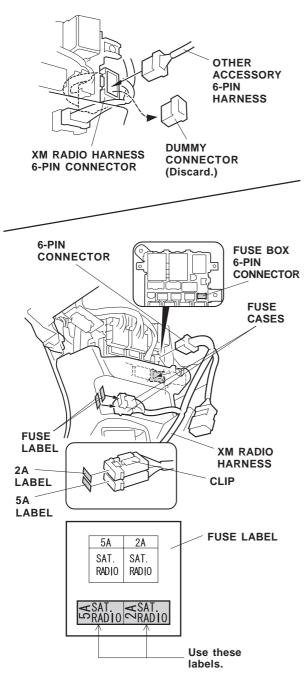
28. Attach the fuse labels to the fuse cases on the XM radio harness.
