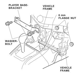
20. On vehicles NOT equipped with a YAW sensor, remove the two 6 mm flange nuts and player base bracket.
