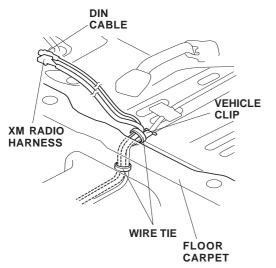
65. Continue to route the XM radio harness and DIN cable along the vehicle harness toward the trunk. Using isopropyl alcohol, thoroughly clean the areas where the cushion tapes will attach, then secure the XM radio harness and DIN cable to the vehicle panel with five cushion tapes.
