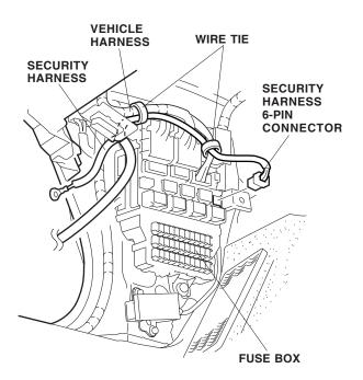
10. Attach the security harness to the vehicle harness with two wire ties.
