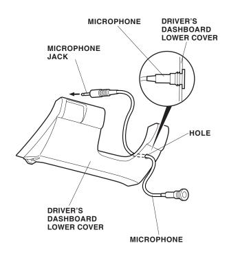
23. Without dashboard under cover: Connect the microphone jack to the security unit, and secure the microphone cord to the vehicle panel with one wire tie. Reinstall the dashboard lower cover. Fold the excess length of the microphone cord, and secure the microphone cord to the security harness with two wire ties.
