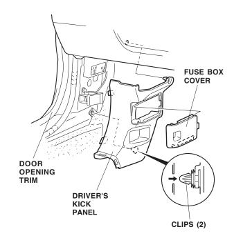
8. Remove the driver's side front door opening trim in the area shown, and remove the driver's kick panel by releasing the two clips.
