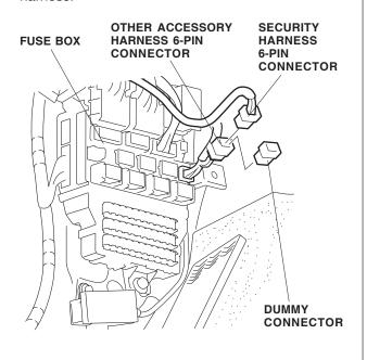
11. Route the ground terminal of the security harness along the vehicle harness. Remove upper bolt from the hood opener, and install the ground terminal using a new ground bolt.
