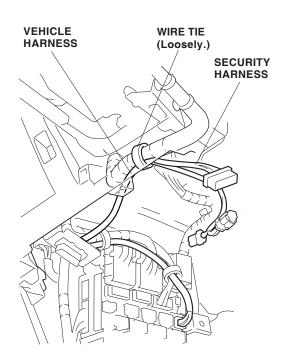
19. On the left of the steering shaft, locate the 3-pin connector blue-taped to the vehicle harness, and connect the security harness 3-pin connector to that 3-pin connector.
