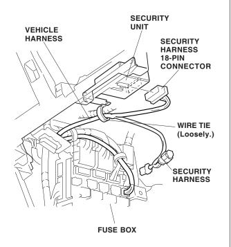
16. *With dashboard under cover:* Slide the security unit into the unit lower cover bracket. Do not push on the connector area.
