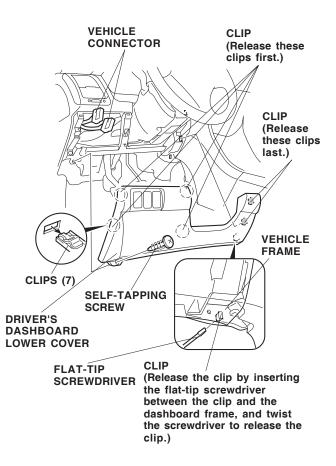
4. If equipped, remove the driver's dashboard under cover (release the three retaining clips, one pin, and one holder).
