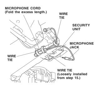
24. *With dashboard under cover:* Measure and fold the excess length of the microphone cord, and secure the microphone cord to the security harness with one wire tie.
