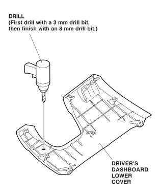
22. Route the microphone jack through the hole you just drilled and secure it.
