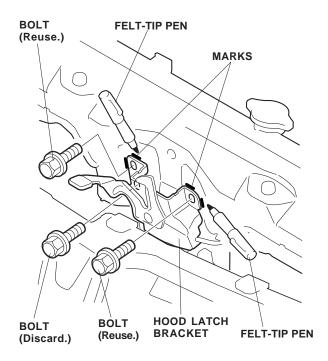
6. Remove the hood latch bracket (three bolts). Discard the one lower bolt shown.
