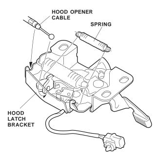
17. Position the hood lock on the center support at the position you marked in step 5. Loosely install the two bolts, and install the hood switch harness ground terminal with the big washer and ground bolt from kit.
