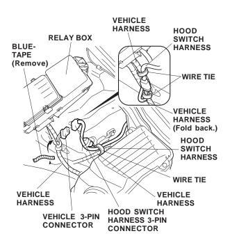
NOTE: If the 3-pin connector is already being used by another accessory, unplug the 3-pin connector. Locate the 3-pin connector taped to the harness. Remove the dummy connector from that harness. Plug the other accessory's harness 3-pin connector into the hood switch harness 3-pin connector. Secure the harness with one wire tie in the area shown.
