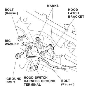
18. Shut the hood, and check that the alignment of the hood lock and the hood latch is correct, and check that the hood is latched securely. When you're satisfied with the results, open the hood, and tighten the hood latch bolts securely.  Route the hood switch harness 2-pin connector along the vehicle harness. Plug the hood switch harness 2-pin connector into the hood switch 2-pin connector.
