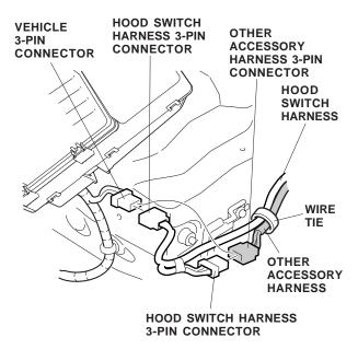
15. Route the hood switch harness along the vehicle harness, and secure it to the vehicle harness with five wire ties in the areas shown.
