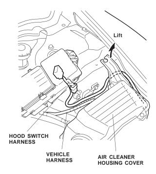
13. Under the relay box, locate the vehicle 3-pin connector blue-taped to the vehicle harness, and remove the blue-tape to free the connector. Connect the hood switch harness 3-pin connector to the 3-pin connector you just freed. Secure the hood switch harness to the vehicle harness with the wire ties.
