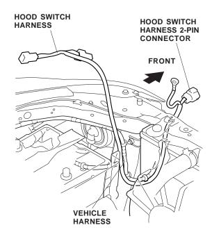
12. Lift the air cleaner housing cover up, and route the hood switch harness to the rear of the air cleaner housing cover along the vehicle harness.
