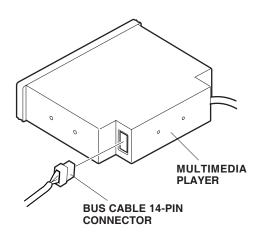
Plug the player BUS cable connector to the vehicle connector, then reinstall the player and pocket.
