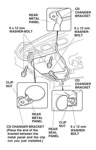
17. Loosely install the 6 x 12 mm washer-bolt to the rear seat panel first. Secure the CD changer bracket to the metal panel with the remaining two 6 x 12 mm washer-bolts. Tighten all three bolts.
