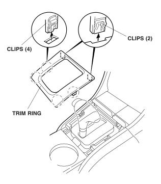
4. Wiggle and then pull up on the cup holder to release the six clips, then remove the cup holder.
