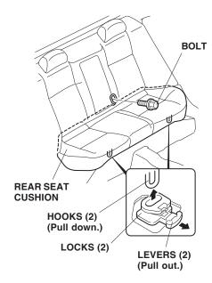
11. Remove the left side cushion (one bolt and two hooks).
