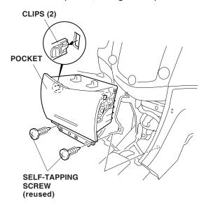
37. Reinstall the player panel using the two screws removed in step 8.
