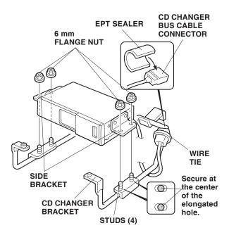
15. Wrap the CD changer BUS cable connector with one EPT sealer, then secure it to the CD changer bracket with one wire tie.
