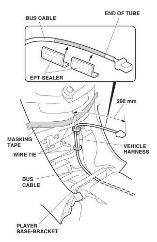
Plug the BUS cable 14-pin connector into the player.
