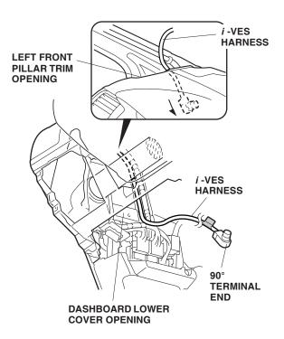
31. Continue routing the 90° end of the *i*-VES harness from the dashboard lower cover opening to the pocket opening on the driver's seat side.
