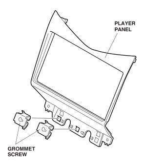
73. Insert the player panel clips into latches, and attach the player panel to the instrument panel with the two self-tapping screws removed in step 10. Remove the masking tape.
