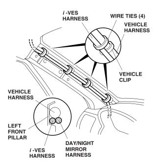
45. Near the fuse box by the driver's dashboard lower cover opening, secure the *i*-VES harness to the vehicle harness with three wire ties in the areas shown.
