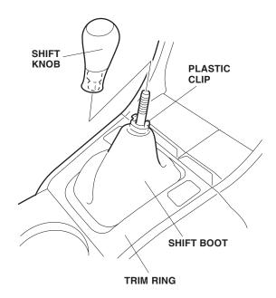
With locknut: Loosen the lock nut and remove the gearshift knob.
