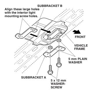
37. Install the two 5 mm plain washers and the subbracket A with the two 5 x 12 mm washer-screws.
