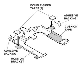
39. Using isopropyl alcohol on a shop towel, clean the vehicle frame where double-sided tapes will attach. Remove the adhesive backings from the double-sided tapes, position the monitor bracket on subbracket A and install the two screws to secure the interior light.
