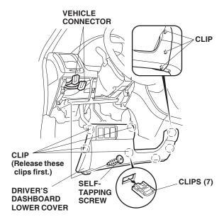
15. If equipped, remove the driver's dashboard under cover (release the three retaining clips, one pin and one holder).
