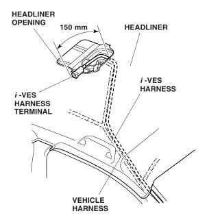
35. Using isopropyl alcohol on a shop towel, clean the area where the cushion tape will attach. Secure the *i*-VES harness to the headliner with the three cushion tapes along with the vehicle harness.
