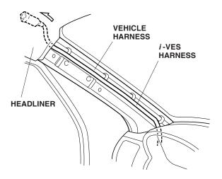
34. Continue routing the *i*-VES harness to the rear along the vehicle harness, and out the opening in the headliner, so that the distance between the headliner opening and end of the *i*-VES harness is 150 mm.
