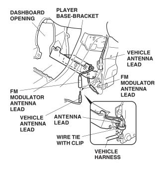
59. Wrap the FM modulator antenna lead and vehicle harness you removed with one wire tie with clip, and push the wire tie with clip into the hole in the player base-bracket. 60. Install the left and right player subbrackets into the holes in the vehicle frame, then install one 6 mm flange nut onto the stud of each subbracket while pushing the player subbracket upward.
