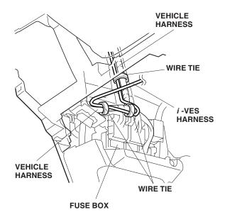
46. Continue to secure the *i*-VES harness to the vehicle harness with the three wire ties in the areas shown.
