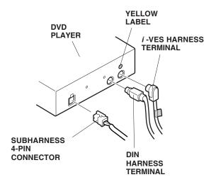
69. Install the DVD player to the brackets using four 6 mm flange nuts.
