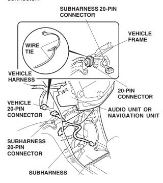
48. Secure the connected 20-pin connectors to the vehicle frame with two wire ties.
