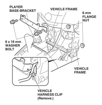
Without YAW sensor: Install the player basebracket to the vehicle frame, then install the two 6 mm flange nuts while holding the bracket firmly against the vehicle frame.
