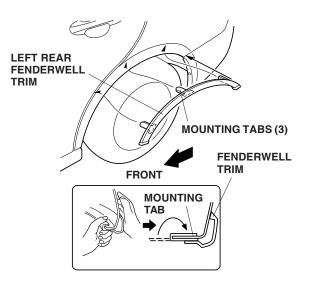
8. Fill the cavity of the inner protector with dishwashing soap and water solution as a lubricant. Starting at the rear of the fenderwell trim drive the inner protector over the fender flange and fenderwell trim using a rubber mallet. Note the direction of the inner protector.
