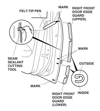
Position the cutting edge of the seam sealant cutting tool against the door edge, and trim the seam sealant from mark to mark, top and bottom.
