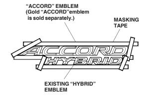
Remove the "HYBRID" emblem from the body by moving the string back and forth, and working it between the emblem and body.
