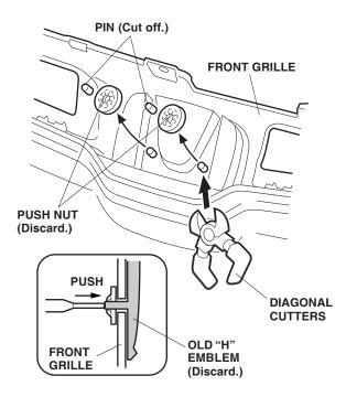
4. Position the gold "H" emblem on the grille by aligning its pins with the holes in the grille.
