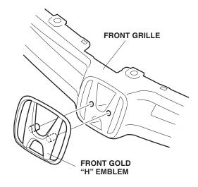
5. Slide the push nuts onto the pins, flat side first. Note the direction of the push nuts.
