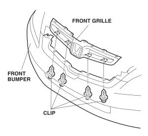
3. Inside the front grille, cut off the two pins, and remove the push nuts and the old "H" emblem.
