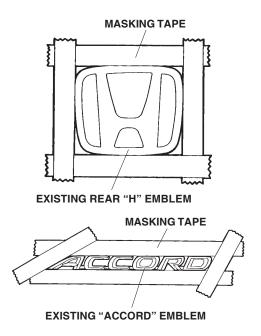
Remove the "H" and "ACCORD" emblems from the body by moving the string back and forth, and working it between the emblems and the body.
