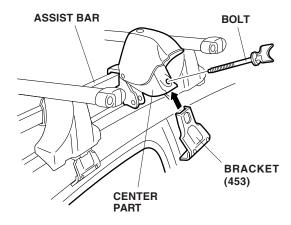
18. Open the locking devices on the center part of the assist bar. Align the center of each rear bracket (marked 453) with the rear recess of the roof by sliding the locking device. Keep the assist bar centered. Close the locking devices.
