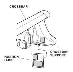
8. Install the rubber pads on the feet of the crossbar support. Each of the four rubber pads has its own location. Before installing the rubber pads, check that the part number shown on the bottom of the rubber pads agrees with those shown in the following table. Check that the pads engage with the feet securely, without lifting.
