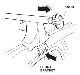
15. Push the knobs on the ends of the front crossbar until they click into position.
