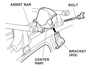
17. Slide the remaining brackets (marked 453) into the center part of the assist bars from the underside and click into position, then loosely install the bolts. Do not tighten the bolts yet.
