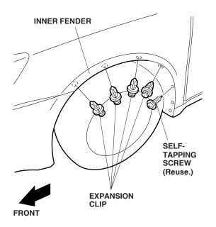
Pull the inner fender down, and position the left front fenderwell trim between the inner fender and the fender flange. Align the fenderwell trim with the front bumper as indicated by the arrow.
