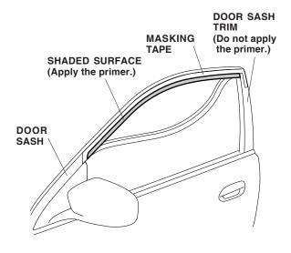
9. Attach the masking tape to the door visor in the area shown.
