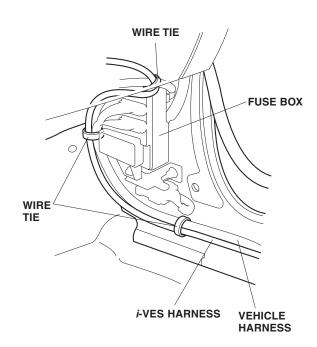
52. In the glove box opening, secure the *i*-VES harness to the vehicle panel with two wire ties.
