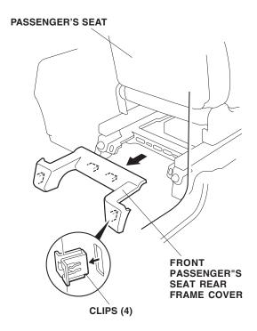
6. Release the four clips, and remove the front passenger's seat front frame cover.
