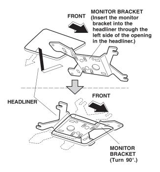
42. Install the monitor bracket to the roof panel with the four 6 x 12 mm washer-bolts.
