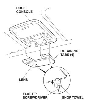
26. Remove the roof console (four screws), and unplug the connector.
