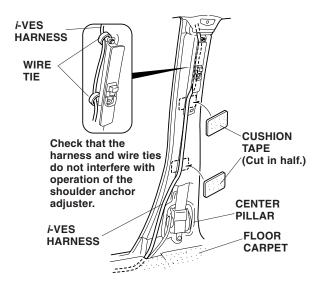
49. Using isopropyl alcohol on a shop towel, thoroughly clean the areas where the cushion tapes will attach. Using scissors, cut the cushion tape in half. Secure the *i*-VES harness to the right center pillar with two pieces of cushion tape in the areas shown.
