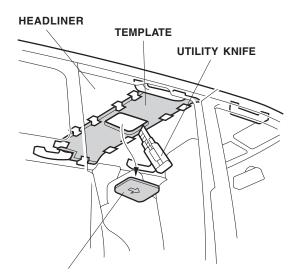
Cut out the marked area of the template along with the headliner.
