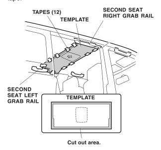
4. Using a utility knife, cut out the marked area from the template along with the headliner as shown.
