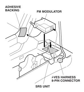
54. Using isopropyl alcohol on a shop towel, thoroughly clean the area where the FM modulator cushion tape will attach. Remove the adhesive backing from the cushion tape, and attach the FM modulator to the SRS unit.
