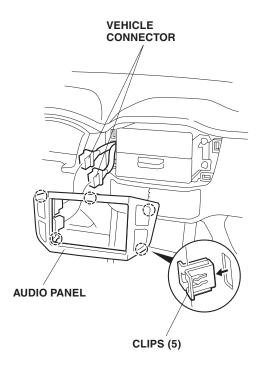
11. Remove the audio unit (four screws, pull the audio unit out toward you; unplug the vehicle connector and antenna lead).
