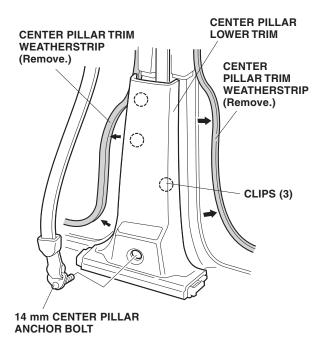
21. Remove the center pillar trim weatherstrip. Pull the center pillar lower trim out toward you to release the three clips, and remove the trim.
