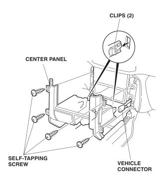
14. Pull the center panel out toward you to release the two clips. Unplug the vehicle connector from the accessory socket, and remove the center panel.
