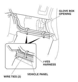
53. In the center console lower cover opening, plug the *i*-VES harness 8-pin connector into the FM modulator.
