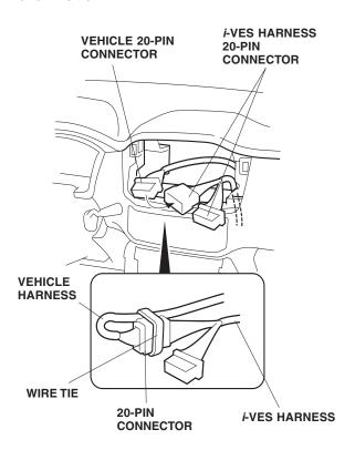
57. Plug the *i*-VES harness 20-pin connector and vehicle antenna lead into the rear of the audio unit. Reinstall the audio unit with the four screws removed in step 11.
