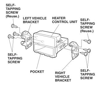
59. Install the DIN bezel to the DVD player. Set the heater control unit on the DVD player, attach the left and right vehicle brackets using the two selftapping screws removed in step 58 and four 5 x 12 mm washer-screws included in the kit.
