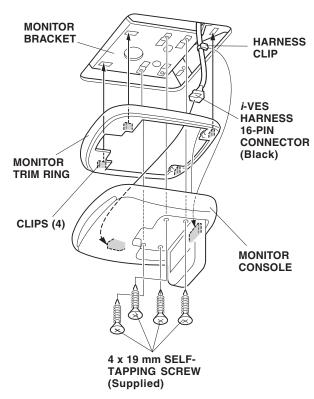
45. Secure the monitor console to the monitor bracket with the four 4 x 19 mm self-tapping screws supplied.
