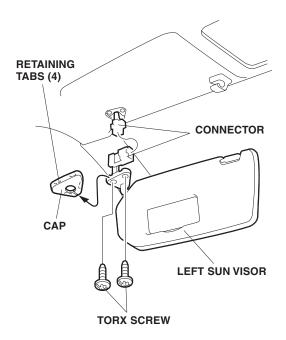
32. Remove the left sun visor (two Torx screws), and unplug the connector.
