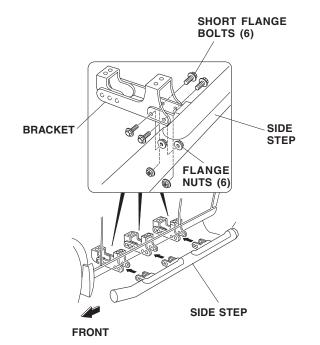
Adjust the location of the left side step so that there is even clearance between the side step and the body, then tighten the long flange bolts installed in step 4. Torque the long flange bolts to 27 N⋅m (20 lb-ft).
