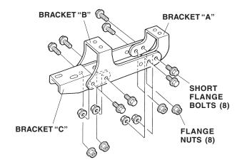
Assemble four center and rear bracket assemblies using brackets "A," "B," and "C" along with 8 short flange bolts and 8 flange nuts. Be sure to use the inboard holes in bracket "B." Do not tighten the nuts or bolts yet.
