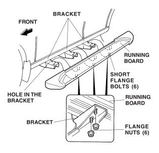
6. Align the rear of the running board with the end of the inner fender, then tighten the long flange bolts you installed in step 4. Torque the long flange bolts to 27 N⋅m (20 lb-ft).
