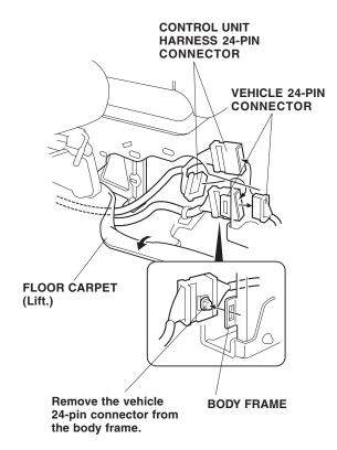
70. Remove the clip that secures the vehicle 24-pin connectors from the body frame. Unplug the vehicle 24-pin connector, and plug in the control unit harness 24-pin connectors in between.
