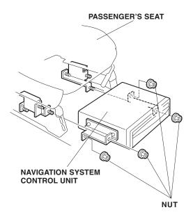
59. Remove the four screws that secure the navigation system control unit bracket.
