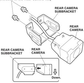
41. Align the two locating tabs on the rear camera subbracket with the slots in the rear camera bracket. Facing the camera, tighten the right side screw using an angle Phillips screwdriver.
