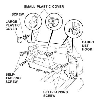
22. Pull the right rear side lining toward you to release the six clips, then unplug the connector at the rear of the right side lining. Remove the lining.
