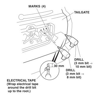
35. Install three rivnuts in the 8 mm holes you just made.
