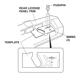
32. To prevent damage, wrap electrical tape around the drill bit at a point about 30 mm away from the tip. While wearing eye protection, drill a 3 mm hole, then a 7 mm hole in 3 places, and finally a 14 mm hole in 1 place. After drilling, remove any burrs from the edges of the holes with a file, and apply touch-up paint.
