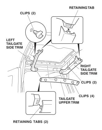
4. Release the one retaining tab and two clips, and remove the right and left tailgate side trims.
