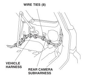
57. Continue routing the rear camera subharness forward and under the passenger's seat, secure it to the vehicle harness with three wire ties.
