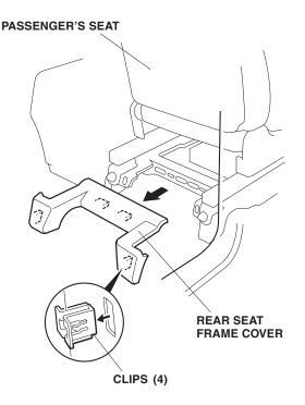
27. Release the four clips, and remove the front seat frame cover from the passenger's seat.
