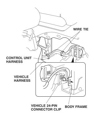
72. Secure the control unit harness to the vehicle harness with two wire ties.
