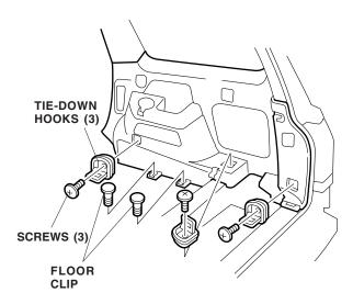
21. Remove the large plastic cover, and remove the screw concealed under the cover. Pry out the two small plastic covers and remove the two self-tapping screws. Tilt the cargo net hooks down, and remove the two self-tapping screws.
