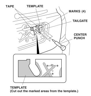
34. Remove the template. To prevent damage to the inner parts, wrap electrical tape around the drill bit 30 mm from the tip. While wearing eye protection drill a 3 mm hole, then an 8 mm hole in 3 places, and finally with a 10 mm hole in 1 place. Remove any burrs from the edges of the holes with a file, and apply touch-up paint. Allow the touch-up paint to dry thoroughly.
