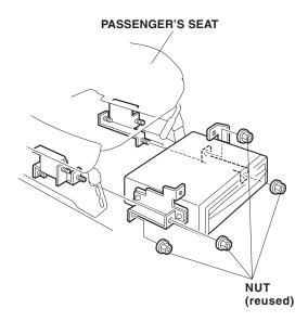
62. Position the two control unit brackets on the sides of the control unit, and install four 5 x 10 mm washer-screws.
