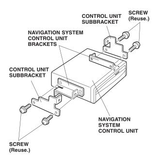
60. Position the two control unit subbrackets and the navigation system control unit brackets on the navigation system control unit, and reinstall the four screws.
