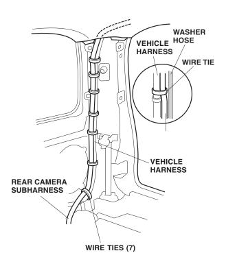
55. Secure the rear camera subharness to the vehicle harness with seven wire ties in the areas shown. Do not attach the wire ties to the windshield washer hose.
