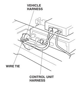
69. Pull the control unit harness out from under the floor carpet.
