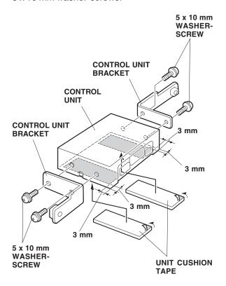
63. Using isopropyl alcohol, clean the areas where the unit cushion tapes will attach. Attach the two unit cushion tapes to the bottom of the control unit in the areas shown.
