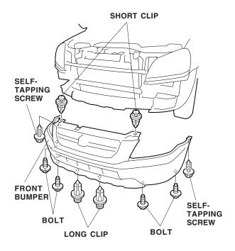
3. Remove ten self-tapping screws, and remove the bumper cover from the front bumper.
