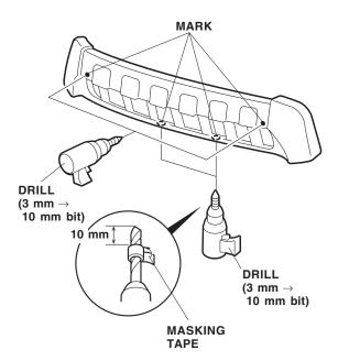
5. Locate two scribed lines on the inside of the bumper cover. Measure 10 mm upward, and 5 mm downward as shown, and mark the bumper with a felt-tip pen.
