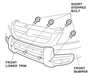
12. Reinstall the front bumper. Make sure that all clips and retaining tabs are attached properly.
