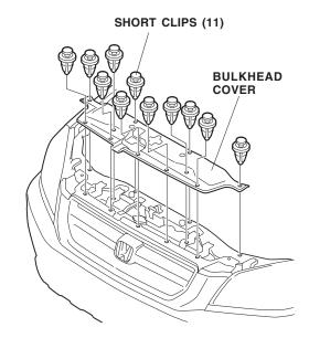
2. Remove two short clips, two self-tapping screws, four bolts and two long clips, then remove the front bumper by pulling it out toward you. To prevent damage, rest the bumper on a blanket.
