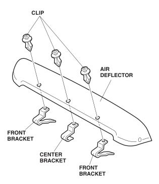
13. Close the hood, and position the air deflector on the hood by sliding the two front brackets and the center bracket over the three protective tapes; align the holes in the air deflector over the two brackets. Install the two 6 x 14 mm screws, the two nylon washers, and two collars, then tighten the screws securely.
