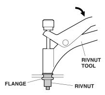
Release the handle, turn the mandrel, and take the tool off the rivnut. 5. Temporarily slide the front brackets over the lip of the hood, and align the hole in the bracket with the hole in the plastic grommets. Install the 5 x 15 mm screw. Repeat on the other side.
