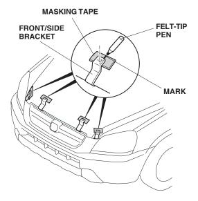
8. Using a felt-tip pen, mark the masking tape where each front bracket and side bracket will rest, then remove the front brackets and side brackets.
