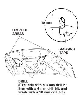
4. Install the two rivnuts into the two holes in the hood using the following procedure:
