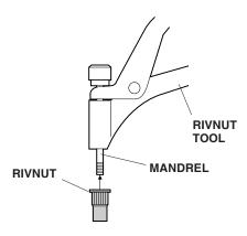
Insert the rivnut into the hole in the body panel.
