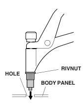
Squeeze the handle firmly until the rivnut is compressed to form a flange-like stopper under the body panel.
