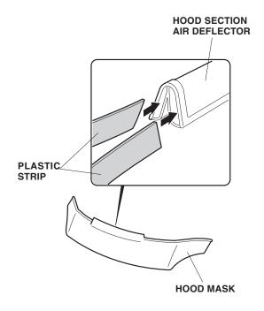
2. Open the hood, fit the corners of the hood section around the hood, and adjust the mask so it fits smoothly over the edges. Attach the seven hooks to the holes in the hood.
