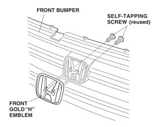
6. Reinstall the front bumper. Check that the clips are installed securely.
