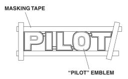
19. Remove the original rear emblem by cutting the outer edges with a piece of string.
