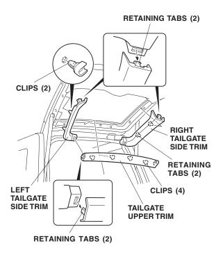
Release the one retaining tab and two clips.
