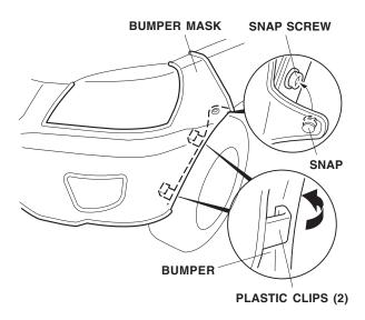
12. Attach the two plastic clips and the four hooks to the bottom corners of the bumper.
