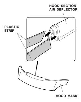
2. Open the hood, fit the corners of the hood section around the hood, and adjust the mask so it fits smoothly over the edges. Attach the seven hooks to the holes in the hood.
