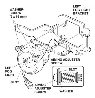
33. On the inside of the front bumper near the hole you cut, remove and discard the two self-tapping screws from the bumper. Position the left fog light bracket on the left mounting bosses, and install two 5 x 20 mm self-tapping screws and one washer to hold the fog light bracket.
