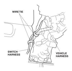
55. Slide the vehicle harness 2-pin connector onto the vehicle connector holder. Secure the switch harness to the vehicle harness with one wire tie as shown.
