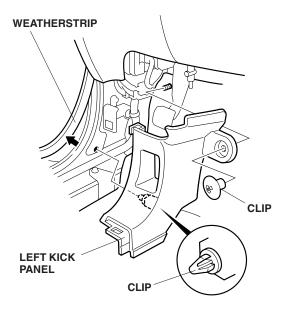
41. Remove the upper clip from the left kick panel, then pull the left kick panel out toward you to release the remaining clip.
