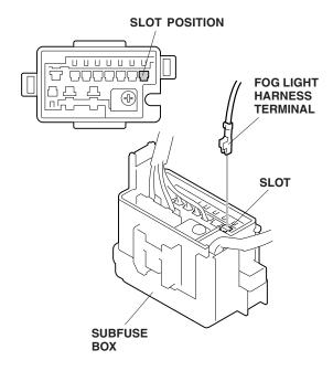
10. Route the fog light harness along the vehicle harness and reinstall the subfuse box under cover.
