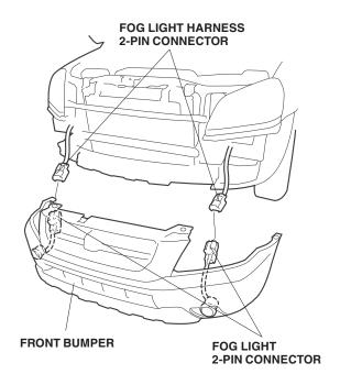
37. On each side, pull the 2-pin connectors out from between the fog light brackets, and slide the 2-pin connectors onto the fog light bracket stays.
