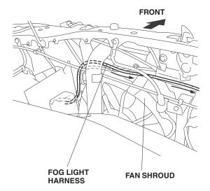
18. Continue routing the fog light harness under the vehicle harness to the right side of the vehicle, then pull the harness out from under the right headlight through the opening near the right horn.
