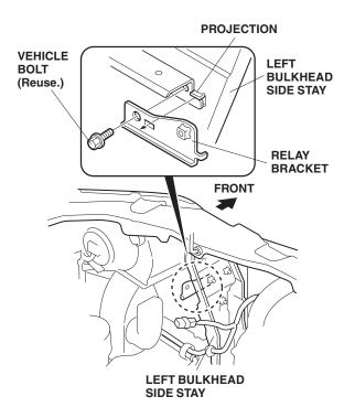
26. Align the projection from the left bulkhead side stay with the hole in the relay bracket and install the relay bracket to the left bulkhead side stay with the vehicle bolt you removed.  Plug the fog light harness 4-pin connector into the relay with rubber cover and install the relay with rubber cover to the relay bracket with one washerbolt.
