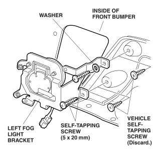
34. Position the left fog light bracket against the front bumper, and install two 5 x 16 mm washer-screws and two collars from the front of the bumper.
