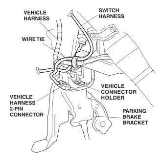
56. Continue to secure the switch harness to the vehicle harness with four additional wire ties in the areas shown.
