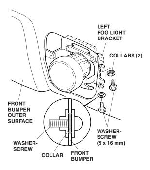
35. Repeat steps 28 through 34 to install the right fog light onto the right fog light bracket at the right side of the front bumper.
