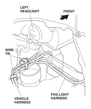
21. At the left front bulkhead panel, secure the fog light harness to the vehicle harness with two wire ties.
