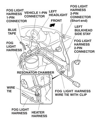
15. Route the other fog light harness 2-pin connector in front of the resonator chamber and secure the wire tie with clip from the fog light harness into the hole in the left bulkhead side stay. If an engine block heater is installed, align the wire tie with clip of the fog light harness with the position of the wire tie attaching the heater harness, and secure the fog light harness to the heater harness with the wire tie.
