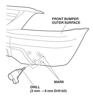
30. Using a 40 mm hole saw, drill through each of the five remaining marks in the front bumper.
