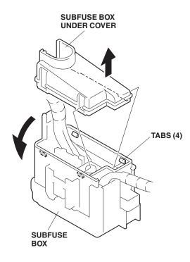
9. Insert the fog light harness terminal into the slot of the subfuse box.
