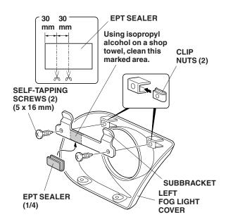
67. Slide the two clip nuts into the openings of the left fog light cover. Position the subbracket on the left fog light cover, and install the two 5 x 16 mm self-tapping screws.
