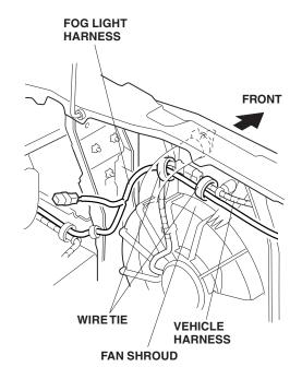
23. Above the right fan shroud, secure the fog light harness to the vehicle harness with five wire ties.
