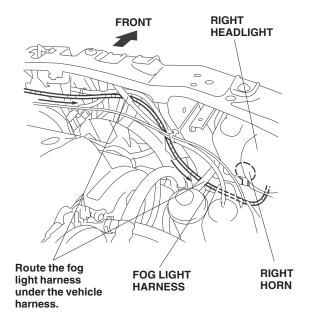
Secure the fog light harness to the vehicle harness with two wire ties.
