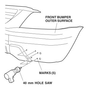
31. On the inside of the front bumper, use a ruler and felt-tip pen to make a line between the corners of the five holes. Using a hacksaw blade, cut out the marked area from the front bumper along the lines. Remove any burrs from the edge of the holes.
