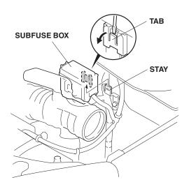
8. Turn the subfuse box upside down and remove the subfuse box under cover (4 tabs).
