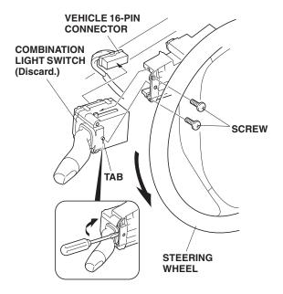
50. Turn the steering wheel in the counterclockwise direction, remove the two screws, disengage the tab of the combination light switch and pull the switch out.
