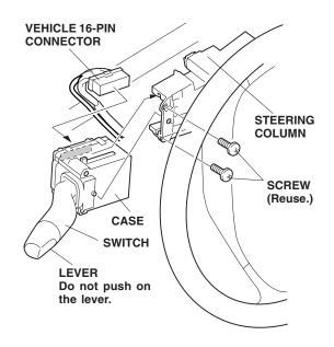
53. Plug the vehicle 16-pin connector into the switch.
