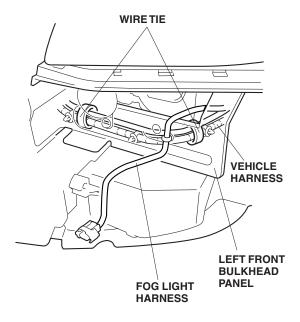
22. Above the left fan shroud, secure the fog light harness to the vehicle harness with two wire ties.
