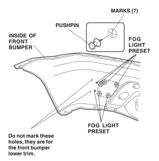
29. While wearing eye protection, drill a 9 mm through each of the two outboard marks you made. Drill from the outer surface inward, first with a 3 mm drill bit, and finish with a 9 mm drill bit. Remove any burrs from the edges of the holes with a file.
