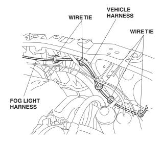
24. Below the right headlight, secure the fog light harness to the vehicle harness with two wire ties.
