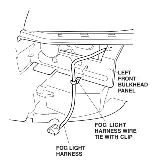
17. Route the fog light harness alongside the vehicle harness and above the fan shroud toward the right (passenger's) side of the vehicle.
