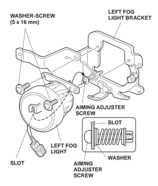
34. On the inside of the front bumper near the hole you cut, remove and discard the two self-tapping screws from the bumper. Position the left fog light bracket on the left mounting bosses, and install two 5 x 20 mm self-tapping screws and one washer to hold the fog light bracket.
