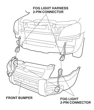
39. On each side, pull the 2-pin connectors out from between the fog light brackets, and slide the 2-pin connectors onto the fog light bracket stays.
