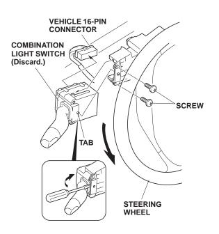
52. Turn the steering wheel in the counterclockwise direction, remove the two screws, disengage the tab of the combination light switch and pull the switch out.
