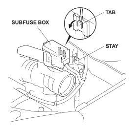
8. Turn the subfuse box upside down and remove the subfuse box under cover (4 tabs).
