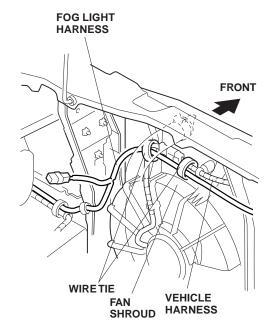
23. Above the right fan shroud, secure the fog light harness to the vehicle harness with five wire ties.
