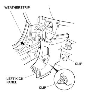
43. Remove the upper clip from the left kick panel, then pull the left kick panel out toward you to release the remaining clip.
