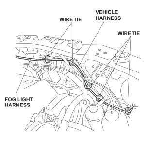
24. Below the right headlight, secure the fog light harness to the vehicle harness with two wire ties.
