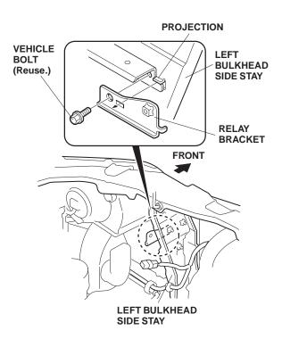
26. Align the projection from the left bulkhead side stay with the hole in the relay bracket and install the relay bracket to the left bulkhead side stay with the vehicle bolt you removed. 27. Plug the fog light harness 4-pin connector into the relay with rubber cover and install the relay with rubber cover to the relay bracket with one washerbolt.
