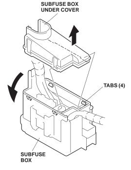
12. Remove the subfuse box cover and insert the fuse (20A) into the subfuse box.
