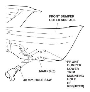
32. On the inside of the front bumper, use a ruler and felt-tip pen to make a line between the corners of the five holes. Using a hacksaw blade, cut out the marked area from the front bumper along the lines. Remove any burrs from the edge of the holes.
