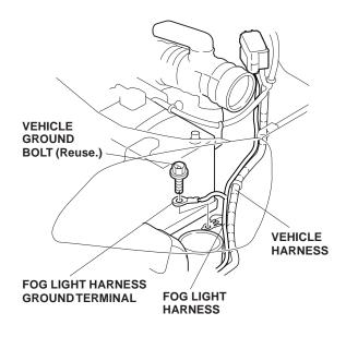
14. Pull the short end of the fog light harness 2-pin connector out from under the left headlight. Under the left headlight, locate the 1-pin connector blue-taped to the vehicle harness. Remove the blue tape to free the connector. Plug the vehicle 1-pin connector into the fog light harness 1-pin connector.
