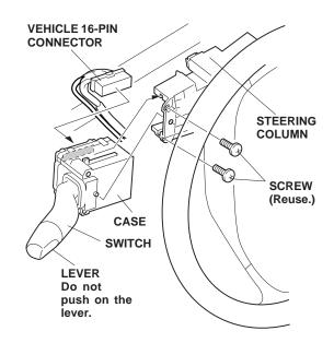
55. Plug the vehicle 16-pin connector into the switch.
