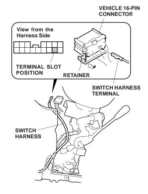
54. Slide the switch onto the steering column and secure the switch with the two screws removed in step 52. Hold the switch case against the column while tightening the screws. Push on the lever.
