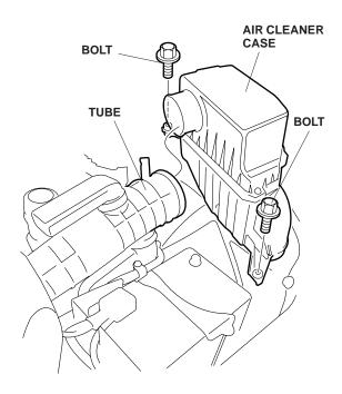
6. Remove the air cleaner case (2 bolts). Be careful not to damage the vehicle harness.
