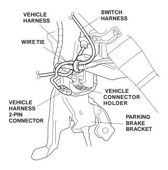
58. Continue to secure the switch harness to the vehicle harness with four additional wire ties in the areas shown.
