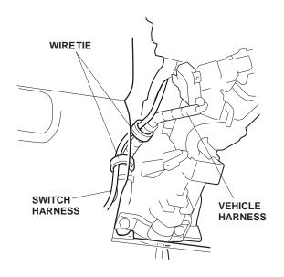
57. Slide the vehicle harness 2-pin connector onto the vehicle connector holder. Secure the switch harness to the vehicle harness with one wire tie in the area shown.
