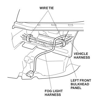
22. Above the left fan shroud secure the fog light harness to the vehicle harness with the two wire ties.
