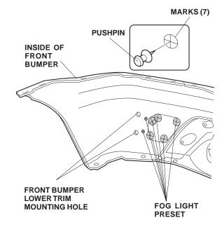
30. While wearing eye protection, drill a 9 mm through each of the two outboard marks you made. Drill from the outer surface inward, first with a 3 mm drill bit, and finish with a 9 mm drill bit. Remove any burrs from the edges of the holes with a file.
