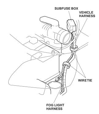
20. Near the left headlight secure the fog light harness to the vehicle harness with two wire ties.
