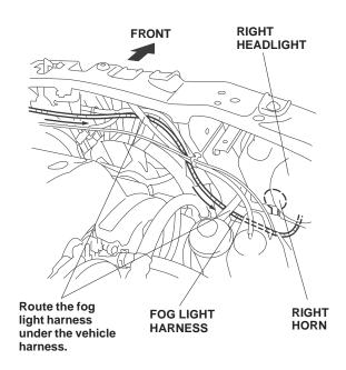
19. Secure the fog light harness to the vehicle harness with two wire ties.
