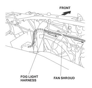
18. Continue routing the fog light harness under the vehicle harness to the right side of the vehicle, then pull the harness out from under the right headlight through the opening near the right horn.
