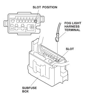
10. Route the fog light harness along the vehicle harness and reinstall the subfuse box under cover.
