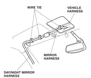
28. *Without RES:* Using isopropyl alcohol on a shop towel, thoroughly clean the areas where the cushion tapes will attach. Secure the day/night mirror harness to the left front pillar with three cushion tapes.
