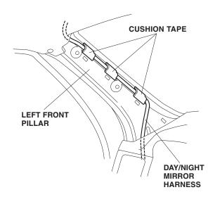
29. *With RES:* After the vehicle harness is routed along the left front pillar, secure the day/night mirror harness to the vehicle harness with three wire ties in the areas shown.
