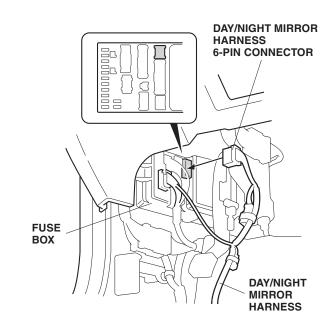
NOTE: If you are also installing the fog lights, remove the dummy connector from the 6-pin connector taped to the day/night mirror harness. Connect the 6-pin connector of the fog light to the 6-pin connector you just unplugged as shown.
