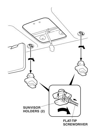
7. Remove the cap from the left sunvisor (four retaining tabs).
