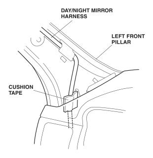
31. Secure the day/night mirror harness to the vehicle harness with three wire ties in the areas shown.
