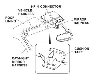
26. Connect the day/night mirror harness 3-pin connector to the 3-pin connector of the mirror harness. Wrap one cushion tape around the connectors.
