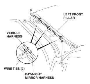
30. Using isopropyl alcohol on a shop towel, clean the area where the cushion tapes will attach. Secure the day/night mirror harness to the left front pillar with one cushion tape in the area shown.
