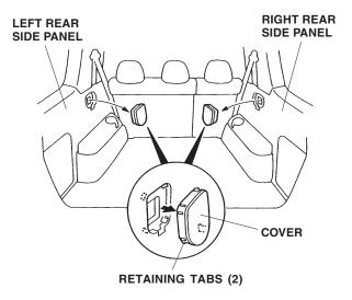
6. Install the cargo cover into the recess in the left rear side panel in the direction shown, then compress the cargo cover, and install it in the right rear side panel.
