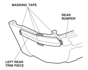
17. Attach a strip of masking tape to the ends of the adhesive backings as shown; remove 5 to 6 inches from the ends. Fold the ends up, and tape them to the front of the trim piece. Remove the remaining adhesive backing.
