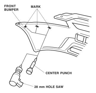
4. While wearing eye protection, drill a 28 mm hole through each of the center-punched marks. Remove any burrs from the edges of the holes with a file. 5. Place the left front trim piece on the front bumper, and adjust it until it fits snugly. Using strips of masking tape, mark the location of the trim piece.
