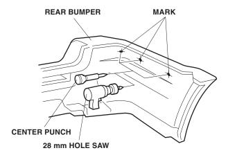
15. While wearing eye protection, drill a 28 mm hole through each of the center-punched marks. Remove all burrs from the edges of the holes with a file. 16. Position the left rear trim piece on the rear bumper, and adjust it until it fits snugly. Using strips of masking tape, mark the location of the trim piece.
