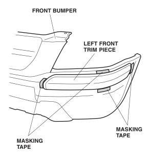
Attach a strip of masking tape to the ends of the three adhesive backings shown; remove 2 to 3 inches from the ends. Fold the ends up, and tape them to the front of the trim piece. Remove the remaining three adhesive backings.
