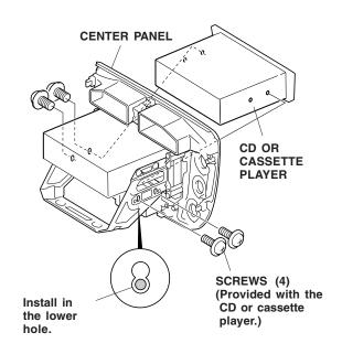
18. Attach the harness clip to the rear of the CD or cassette player with the washer-screw provided.
