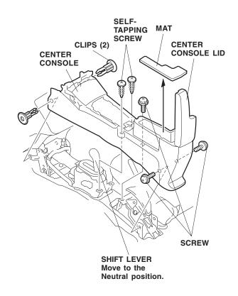
9. Remove the two clips, two self-tapping screws and three screws that fasten the center console. Move the shift lever to the Neutral position, and remove the center console.
