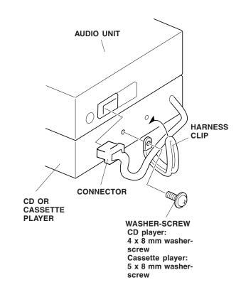
19. Plug the connector from the CD or cassette player into the rear of the audio unit, and secure the harness with the harness clip.
