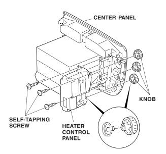
12. Remove the three self-tapping screws that fasten the heater control panel to the center panel, and remove the heater control panel. 13. Remove the pocket (four self-tapping screws).
