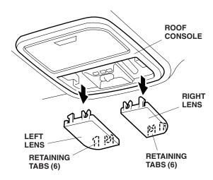
4. Remove the roof console (four bolts, and unplug two connectors).
