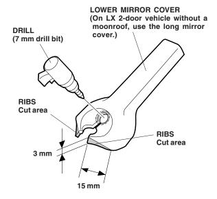
9. While wearing eye protection, drill a 7 mm hole through the existing hole on the lower cover as shown.
