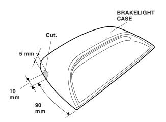
69. Route the antenna cable through the groove in the high mount brake light case, and reinstall the high mount brake light case.
