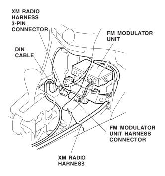
39. Unplug the vehicle antenna cable, and plug it into the FM modulator unit antenna cable. Plug the other end of the FM module antenna jack into the vehicle antenna cable.
