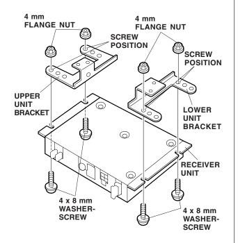
75. Position the receiver unit between the right trunk side panel and the rear fender panel, and plug in the antenna cable connectors, the DIN cable connector, and the XM radio harness connector using the panel hole to access the receiver unit.
