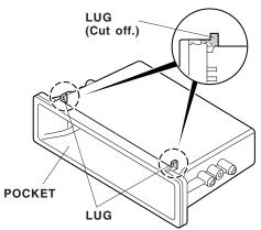
11. Install one latch onto the left and right player brackets. Slide the clip nut onto the display module pocket flange.
