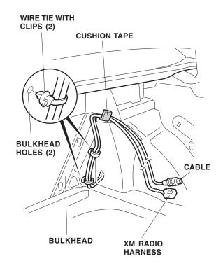
64. Using isopropyl alcohol on a shop towel, clean the area where the cushion tape will attach. Attach the DIN cable and XM radio harness to the vehicle frame with one cushion tape.
