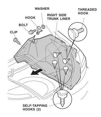
58. Remove the right side trunk liner (three self-tapping hooks, one threaded hook and one clip).
