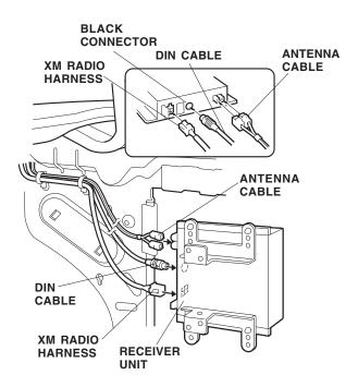
76. Secure the antenna cable, the XM radio harness, and the DIN cable with two wire ties with clip at the measurement shown. Press the clips of the wire ties into the trunk side panel hole and upper unit bracket hole.
