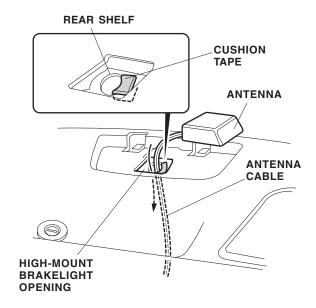
66. Temporarily fit the high-mount brake light onto the rear shelf.
