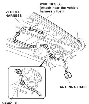
VEHICLE HARNESS CLIP 71. Attach one wire tie with clip to the antenna cable, the XM radio harness and the DIN cable in the area shown. Push the clip from the wire tie with clip into the body hole.
