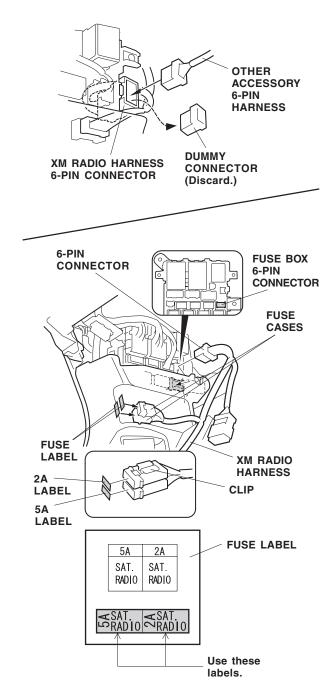
26. Attach the fuse labels to the fuse cases on the XM radio harness.
