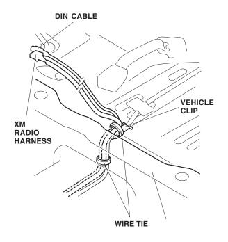
61. Continue routing the XM radio harness and DIN cable along the vehicle harness toward the trunk. Using isopropyl alcohol, clean the areas where the cushion tapes will attach, then secure the XM radio harness and DIN cable to the vehicle panel with five cushion tapes.
