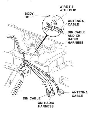
72. Route the antenna cable, the XM radio harness, and the DIN cable along the trunk side panel. Loosely attach the three off-set wire ties with clip around the antenna cable, the XM radio harness, and the DIN cable, then push the clip from each wire tie into the three holes in the trunk side panel.
