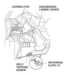
23. If equipped, remove the driver's dashboard under cover (release the three retaining clips, one pin, and one holder).
