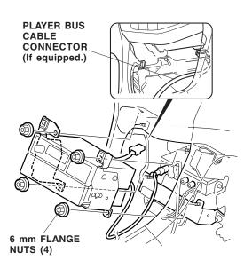
44. Install the display module assembly onto the studs from the left and right player subbrackets, and install the 6 mm flange nuts. Tighten the flange nuts securely.
