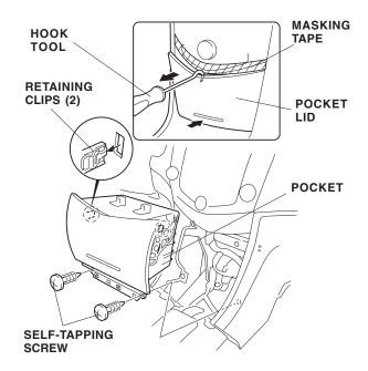
6. Remove the right and left inner covers (one hook and one clip for each cover). Set the inner covers aside; they will not be reused.
