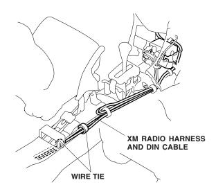
60. Raise the rear seat back. Pull the XM radio harness and DIN cable out from under the floor carpet and toward the passengers' side of the vehicle. Secure the XM radio harness and the DIN cable to the vehicle harness with two wire ties.
