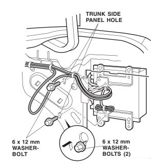
79. Fold any excess antenna cable, and wrap the excess cable with two EPT sealers. Secure the antenna cable to the XM radio harness with two wire ties in the areas shown. Tighten the off set wire ties you loosely installed in step72.
