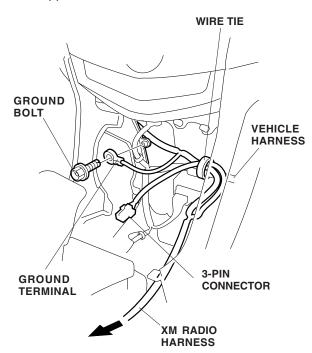
31. Secure the XM radio harness to the vehicle harness with one wire tie. Route the 3-pin connector, and the remaining end of the XM radio harness toward the rear of the vehicle; they will be routed later.
