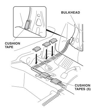
62. Using isopropyl alcohol, clean the bulkhead area where the cushion tape will attach. To prevent damage to the XM radio harness and DIN cable, attach the cushion tape to the bulkhead edge in the area shown. 63. Inside the trunk, install the two wire ties with clip to the DIN cable, and XM radio harness, and push the clips into the holes in the bulkhead.
