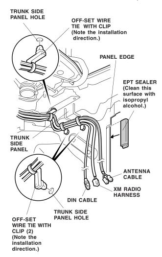
73. Using isopropyl alcohol on a shop towel, clean the bonding surface on the panel edge, attach one EPT sealer to the panel edge in the area shown.
