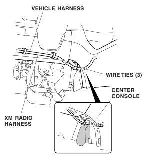
29. Loosely attach the XM radio harness to the vehicle harness with three wire ties.
