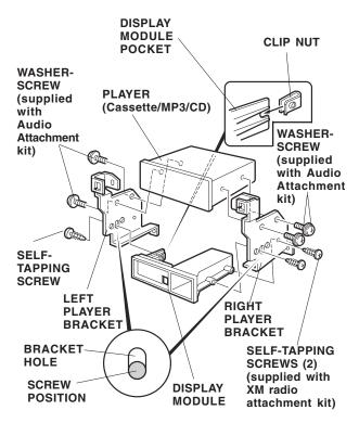
17. Set the player on the display module pocket. Position the left and right player brackets on the display module pocket and player, and reinstall the four washer-screws. Install the three self-tapping screws to secure the display module pocket.
