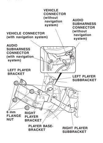
15. Remove the left and right audio brackets (two washer-screws and one self-tapping screw for each bracket). Separate the player and pocket. Set the pocket aside; it will not be reused.
