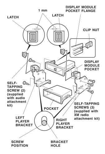
12 Set the display module pocket on the pocket with the cut out facing up. Position the left and right player brackets on the display module pocket and pocket, and install five self-tapping screws.
