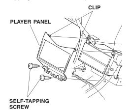
14. Remove the player/pocket assembly. Unscrew the four flange nuts, and pull the assembly out toward you. Unplug the audio subharness cable connector.
