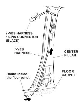
31. Wrap the piece of wire around the *i*-VES harness 16-pin connector. Using electrical tape, secure the wire to the connector so that the end of the wire will not get caught. Pull the 16-pin connector behind the headliner and out of the small cutout until the harness clip comes through the cutout. Remove the tape and the wire.
