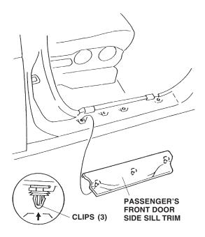
15. Peel up the door opening trim, and remove the passenger's kick panel (one plastic screw and one clip).
