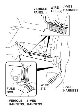
39. In the glove box opening, secure the *i*-VES harness to the vehicle panel with two wire ties.
