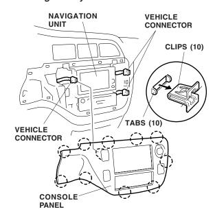
Remove the audio unit (four bolts, and unplug the vehicle connector and the antenna lead). If equipped, remove the navigation unit (two selftapping screws and four bolts, and unplug the vehicle connectors and the antenna lead).
