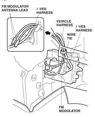
46. Plug the vehicle antenna lead into the FM modulator antenna lead.
