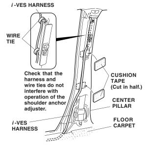
36. Using isopropyl alcohol on a shop towel, thoroughly clean the areas where the cushion tapes will attach. Using scissors, cut the cushion tape in half. Secure the *i*-VES harness to the center pillar with the two pieces of cushion tape in the areas shown.
