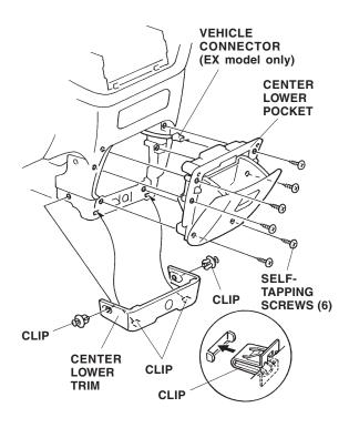
Open the center lower pocket, and remove the six self-tapping screws. Disconnect the vehicle connector (if equipped), and remove the center lower pocket. 11. Disconnect the accessory socket from the accessory socket harness connector, then remove the socket from the instrument panel by unscrewing the socket from the socket holder.
