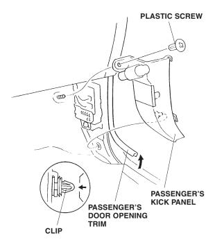
16. On the passenger's side of the vehicle, remove the sliding door sill trim (lift up to release the five clips).
