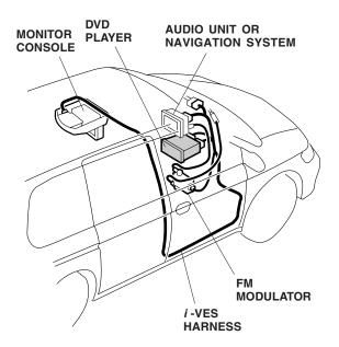
Illustration of the DVD Player installed in the audio unit opening (pocket equipped).
