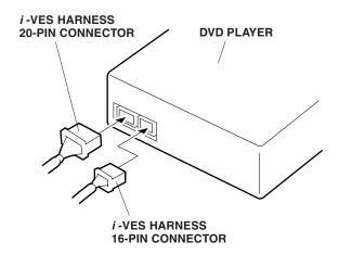
49. Slide the DVD player into the beverage holder opening, and install the three self-tapping screws and two screws you removed in step 13, along with the two 5 mm flange nuts provided. Do not pinch the vehicle harness between the DVD player bracket and the vehicle frame.
