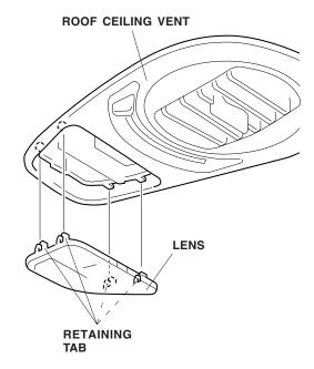
26. Move the vent knob to the closed position, then remove the two screws that fasten the roof ceiling vent. Unplug the vehicle connector, and remove the roof ceiling vent.
