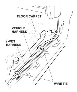
38. Near the fuse box, secure the *i*-VES harness to the vehicle harness with one wire tie. Make sure you do not secure the *i*-VES harness to the yellow SRS harness.
