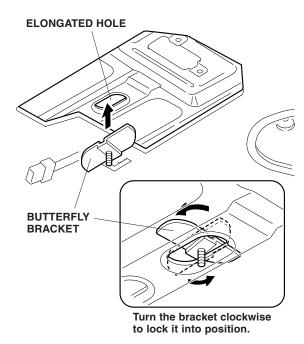
33. Position the monitor bracket on the roof panel, install the locknut onto the butterfly bracket, and install the two 5 x 12 mm washer-screws. Tighten the locknut and the washer-screws securely.
