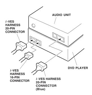
55. Slide the audio unit and DVD player into the audio unit opening, and install the four bolts.
