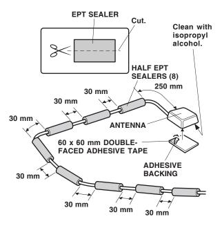
12. Using isopropyl alcohol on a shop towel, clean the bottom of the antenna unit. Remove the adhesive backing from one side of the 60 x 60 mm double-sided adhesive tape, and attach it to the bottom of the antenna.
