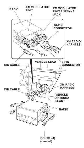
44. Reinstall the radio (four bolts; reused).
