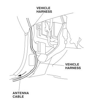
22. Turn over the floor carpet. From the rear of the fuel lid opener, route the antenna cable under the floor carpet and out through the opening in the floor carpet.
