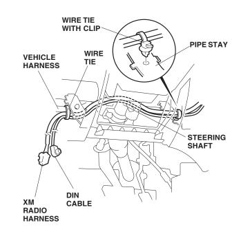
41. Secure the XM radio harness and DIN cable to the pipe stay with the one wire tie with clip. Push the clip of the wire tie into the pipe stay hole. Secure the harness and cable to the vehicle harness with one wire tie in the area shown.
