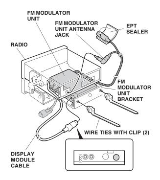
36. Loop the FM modulator cable and the display module cable and wrap it with the two wire ties with clip.
