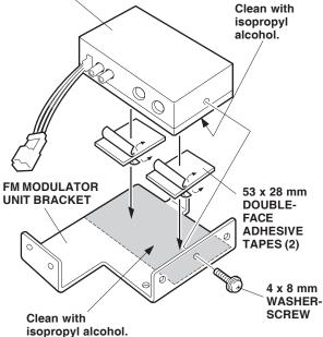
29. Press the FM modulator unit into place, and then install the FM modulator unit onto the bracket with 4 x 8 mm washer-screw.
