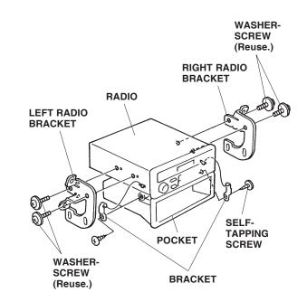
26. Install the left and right radio brackets (two washer-screws for each bracket.)
