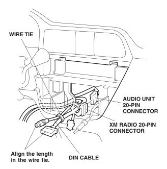
39. Route the DIN cable along the XM radio harness, and align the DIN connector with the XM radio 20-pin connector. Secure the DIN cable and the XM radio harness with one wire tie in the area shown. 40. Route the XM radio harness and DIN cable over the pipe stay, the steering shaft, and toward the driver's under-dash fuse/relay box.
