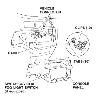
4. Remove the radio (remove the bolts, and unplug the vehicle connector and the antenna lead).
