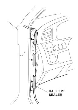
21. Route the antenna cable along the vehicle harness.
