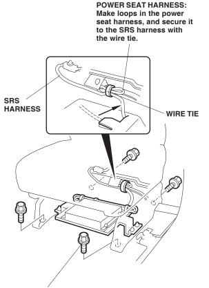
BOLTS (4) (reused) Torque to 41 to 53 N·m (30.4 to 39.1 lb·ft)
