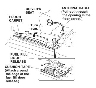
23. Using isopropyl alcohol on a shop towel, thoroughly clean the edge of the fuel fill door release where the cushion tape will attach. Remove the adhesive backing from the cushion tape, and attach it to the edge of the fuel fill door release.
