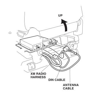
48. Using two wire ties with clip and two wire ties, secure the XM radio harness, the DIN cable, and the antenna cable in the areas shown. Push the two wire ties with clip into the holes in the receiver unit bracket.
