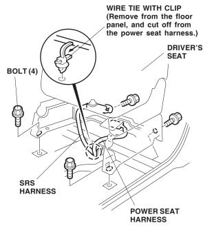
• Under the driver's seat, mark the floor carpet as shown. Using a utility knife, make a cut in the floor carpet as indicated by the mark.
