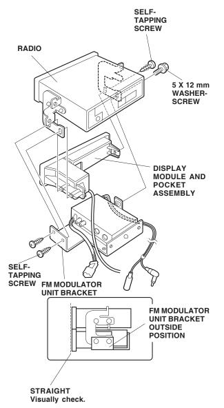
35. Plug the display module cable into the FM modulator unit. Plug the FM modulator unit antenna jack into the radio. Wrap one EPT sealer around the other antenna cable jack. Insert the clips of the two wire ties with clip into the holes in the FM modulator unit bracket.
