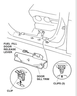
6. Pry up on the clips, and remove the driver's side front door sill trim. Be careful not to damage the clips.
