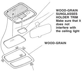
ADHESIVE BACKING Remove one inch of adhesive backing from the end of each adhesive tape, and tape them to
