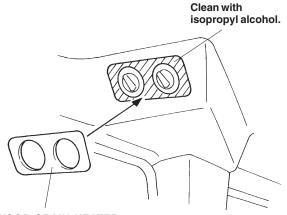
WOOD-GRAIN HEATER CONTROL PANEL TRIM Remove the adhesive backing before attaching.
