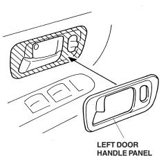
HANDLE PANEL (Remove all the adhesive backings before attaching.)
