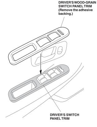
Remove the adhesive tape backings from the passenger's side wood-grain switch panel trim. Carefully position wood-grain switch panel trim on the switch panel. Using the palm of your hand, apply pressure on the wood-grain switch panel trim for about 30 seconds
