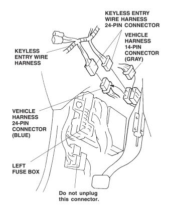
10. Unplug the 6-pin and 10-pin connectors from the left fuse box, and plug the 6-pin and 10-pin connectors from the keyless entry wire harness in between.
