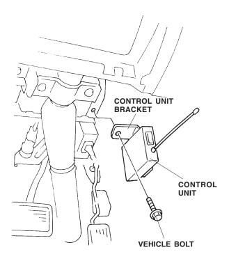
20. Attach the wire tie with clip to the control unit antenna, and push the clip into the hole in the instrument panel.
