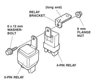
16. Under the dash, remove the nut securing the ABS unit, and attach the relay bracket. Reinstall the nut.
