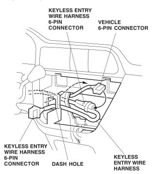
23. Route the 6-pin connector of the keyless entry wire harness out the dash hole.
