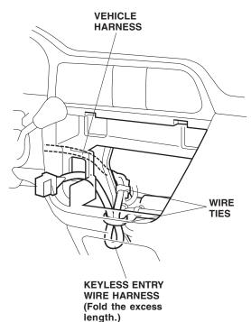
25. Under the dash, secure the keyless entry wire harness to the vehicle harness with six wire ties in the areas shown.
