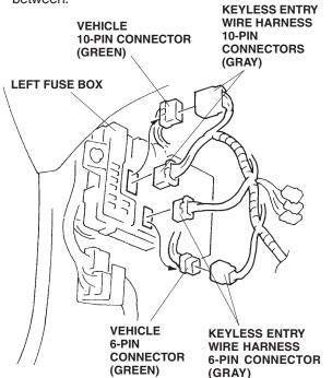
11. Locate the gray 3-pin connector blue-taped to the vehicle harness, and remove the tape to free the connector. Connect the 3-pin connector to the 3-pin connector of the security system wire harness.
