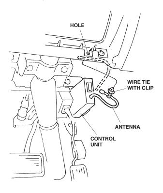
21. Plug the keyless entry wire harness 22-pin connector into the control unit.
