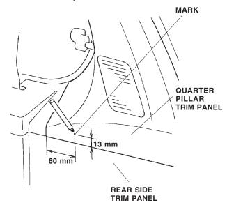
3. On one side of the cargo area, measure 25 mm toward the front from the rear end of the quarter pillar trim panel, and 13 mm up from the rear side trim panel. Mark the spot with a water-soluble pen. Repeat the measurement and mark the spot on the other side of the cargo area.
