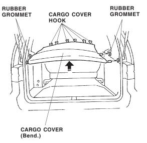
7. Attach the six cargo cover hooks to the rear seat headrest stays as shown.
