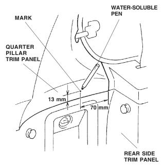
On the right (passenger's) side of the cargo area, measure 60 mm toward the rear from the front corner of the right quarter pillar trim panel, and measure 13 mm upward. Mark the spot with a water-soluble pen.
