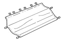
4 Rubber grommets (Replacement grommets: P/N 08U35-S10-100R1)
