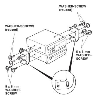
7. Attach the harness clip to the back of the CD player with the remaining 5 x 8 mm washer-screw. Plug the BUS cable into the rear of the radio/cassette player; then fold the excess BUS cable several times, and secure it to the back of the CD player with the harness clip.
