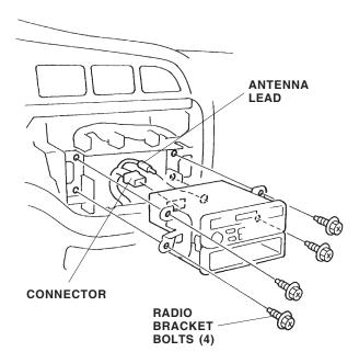
4. Remove the left and right radio brackets (two washer-screws for each bracket).
