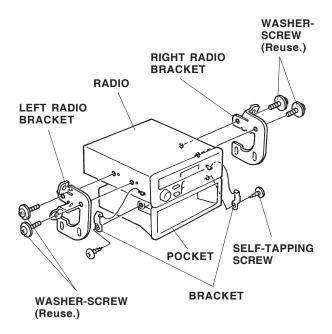
Remove the pocket (two self-tapping screws), then separate the radio and pocket. Set the pocket aside, it will not be used.  Position the CD player on the radio, and reinstall the left and right radio brackets and four washerscrews removed in step 4. Use four 5 x 8 mm washer-screws (supplied) to secure the CD player to the radio brackets.
