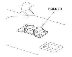
15. Remove the adjusting nut from the quick shaft, then slide the shaft through the pipe on the holder in either direction.
