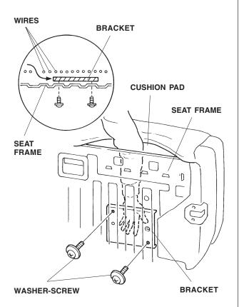
11. Fold the rear seat down, and remove the rear seat handle from the seat.
