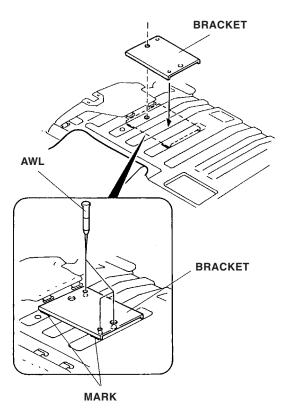
7. While holding the bracket in place, mark the seat frame through the three holes using an awl. Remove the bracket.
