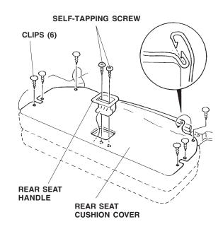
13. While pressing on the rear seat cushion cover with the tip of your finger, locate the two washer-screws you installed in step 10.
