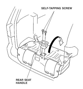
10. Have an assistant hold the seat in the upright position. While wearing gloves, position the bracket between the seat cushion pad and seat frame and install the two washer-screws. You will need to turn the bracket sideways, then fit it between the wires.
