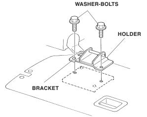
The holders can be installed in two directions, position A or B, according to the type or the number of the bikes to be mounted on the holders. The position of the bike is changed by about 90 mm in longitudinal direction when the direction of the holder is changed.
