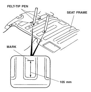
6. Set the bracket on the seat frame at the marks you made in step 5; align the large hole in the bracket over the existing hole in the seat frame.
