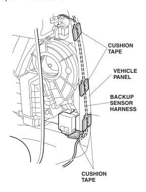
35. Secure the backup sensor harness to the air duct with one long wire tie.
