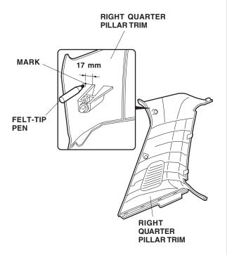
38. While wearing eye protection, drill a 13/16" (20 mm) hole through the mark you just made. Remove any burrs.
