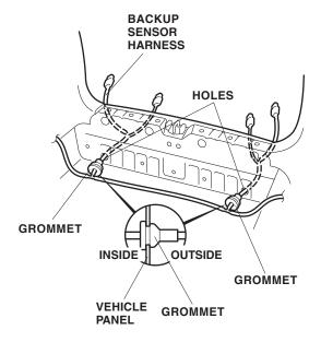
26. From the recess below the tailgate latch, measure 50 mm upward and mark the body. Position the sensor harness on the vehicle panel, and align it with the mark you just made.
