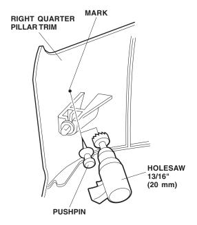
39. Install the two clips on the air duct. Pull the backup sensor harness 4-pin connector out through the 13/16" (20 mm hole) you made, then reinstall the right quarter pillar trim. Check that all clips and retaining tabs are installed securely.
