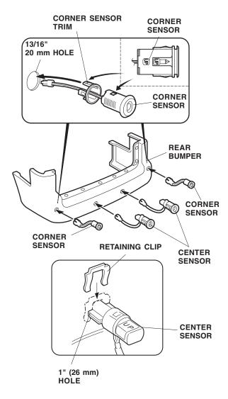
Slide the two center sensors into the 26 mm holes.
