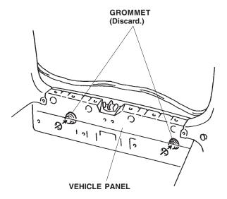
25. Route the backup sensor through the holes in the vehicle panel, and seat the two grommets into the holes.
