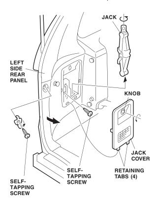
16. Remove the tailgate weatherstrip. Pry up on the two clips and the four retaining tabs, and pull out on the left rear side panel.
