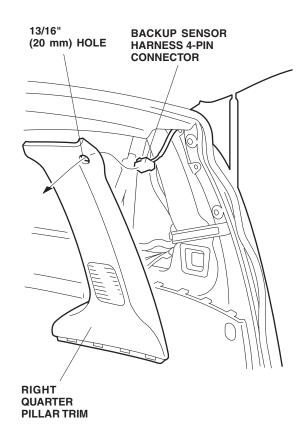
40. Plug the backup sensor harness 4-pin connector into the switch, and install the switch into the hole in the right quarter pillar trim in the direction shown.
