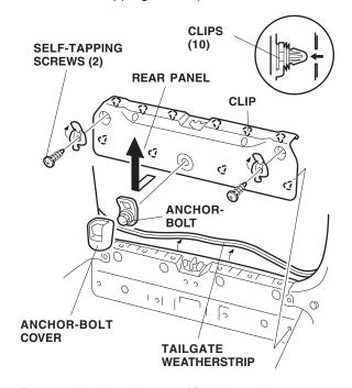
15. Remove the headrest, and fold down the rear seat. Remove the jack cover and the jack (one knob and four retaining tabs). Remove the two self-tapping screws that fasten the left rear side panel.
