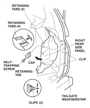
18. Remove the tailgate weatherstrip and the window molding. Pry up on the two clips and the five retaining tabs, and remove the right quarter pillar trim.
