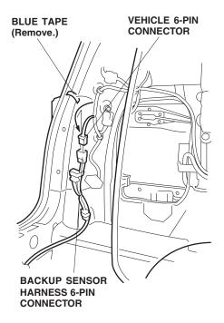
NOTE: If you are also installing a trailer hitch, remove the blue tape to free the 6-pin connector of the backup sensor harness. Connect the trailer hitch 6-pin connector to the 6-pin connector you just freed, and attach a black cushion tape to the backup sensor harness 6-pin connector.
