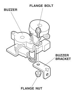
32. Plug the backup sensor harness 5-pin connector into the 5-pin connector of the buzzer.
