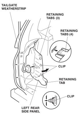
17. Remove the one self-tapping screw that secures the right rear side panel. Remove the tailgate weatherstrip. Pry up on the two clips and the four retaining tabs, and pull out on the right rear side panel.
